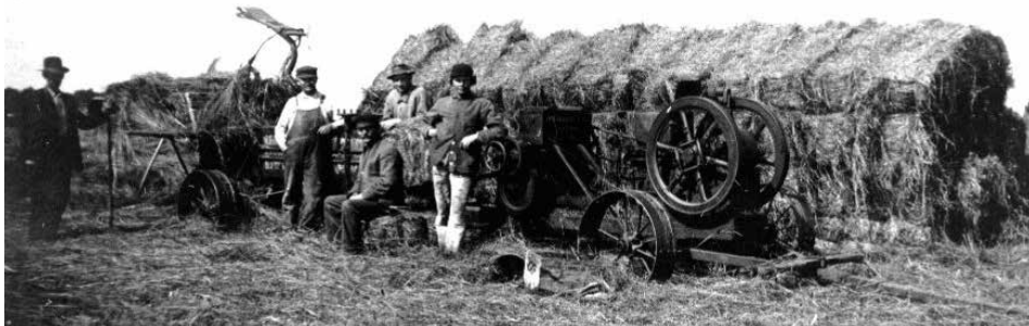
A Lawbaugh photo of creating bales from marsh hay with a steam press. Credit "RTS100"
